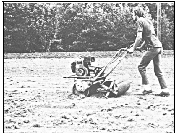
Figure 6. The vertical blades of a Bermuda sprigger slice the stolon into the soil, and the roller then firms the soil around the stolon.
