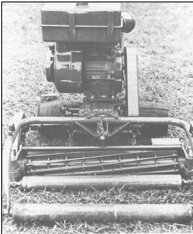
Figure 8. Reel mowers work best on hybrid bermudagrasses and Zoysia. A reel mower with 5 or 6 blades is good for a lawn.
